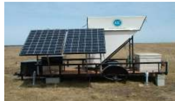
The Wastewater System's SODAR wind profile unit was put in operation in April
