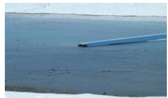
Sludge pumped from Cell #4 flowing into a drying basin
