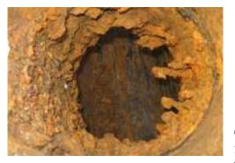
Corrosion inside Quarterline Road water main tee
