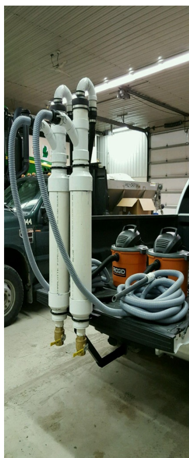
The newly-built seed vacuum system, which makes for easy, fast cleanup of the corn planter.
