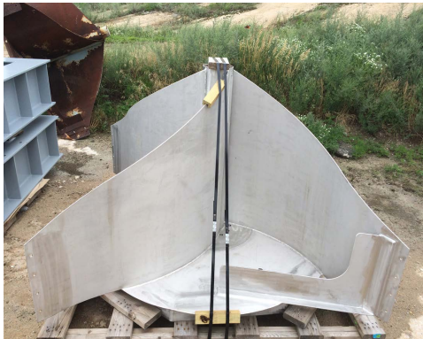
Just arrived for Cell Two: A paddle for the new mixers. For perspective on the size, it's sitting on a 6-foot wooden palette.
